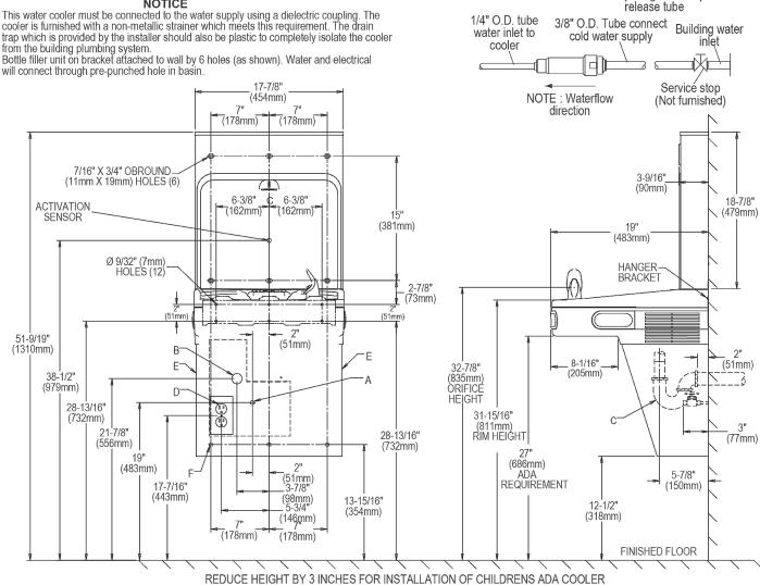
A = Recommended Water Supply location. Shut-off Valve (not furnished) to accept 3/8" O.D. unplated copper tube. Up to 3" (76mm) maximum out from wall.
