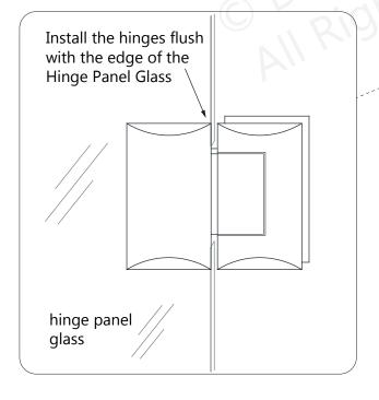
TIP: Clean the hinge gaskets and the glass around the hinge notches with an ammonia-free glass cleaner before installing the hinges onto the glass.
