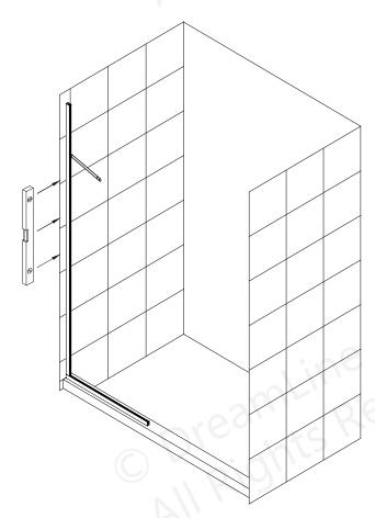
**14.** Add several 2" pieces of the **PVC Glass Spacer (0.5mm) (#34)** into the **Bottom U-channel** to protect the bottom edge and corners of the glass. Apply a good quality mildew-resistant silicone into both U-channels. **(Fig 14)**
