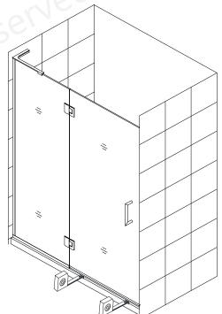
**25.** Apply a good quality mildew-resistant/waterproof silicone along the connection of both U-Channels to the wall and threshold on the inside of the shower.
