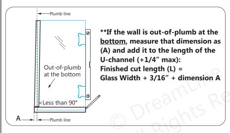
**NOTE** The Vertical U-channel for the <u>Hinge Panel</u> glass will accomodate **up to 1/4**" **for out-of-plumb. Do not exceed this amount.**
