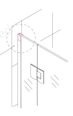
6" Hinge Panel with Hinge Panel Glass Bracket (#36)
