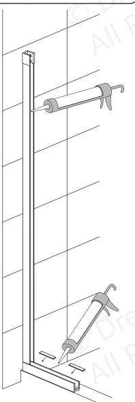
Hinge Panel Glass Bracket with gasket top 7-7/8" bottom, 8-3/8"
