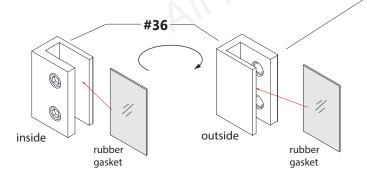
NOTE: The Hinge Panel Glass Bracket (#36) is only to be installed with the 6" Hinge Panel Glass (#32) for the UNIDOOR-X models.
