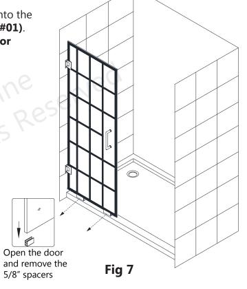
Hold the door in a closed position, parallel to the outside edge of the threshold. Mark the threshold in several places along the U-Channel, checking with a tape measure to stay in-line.
