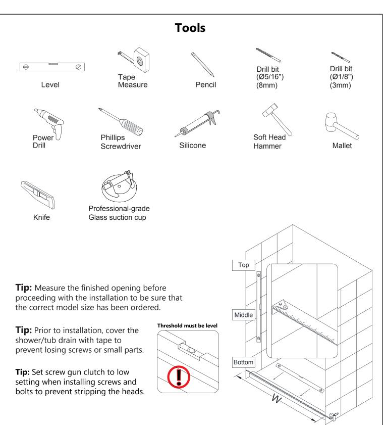
**NOTE:** Unpack your unit carefully and inspect it. Lay it out and identify all parts using the detailed diagram and packing list in this manual as a reference. Before discarding the carton, check for small hardware bags that may have fallen to the bottom of the box. If any parts are damaged or missing, please contact DreamLine<sup>®</sup> for replacement. The shipping boxes may contain extra parts not used in your model configuration.
