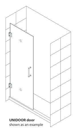
**1.** Align the **Door** so that it is perpendicular to the wall and parallel with the outside of the threshold. Mark a line on the threshold for reference. Open the door to allow space for the panel installation. **(Fig 1)**
