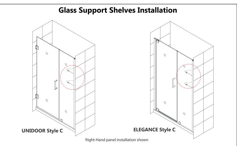
**10.** Mark the **Glass Shelf (#12)** position on the wall. According to the measurements in **Fig. 10a1**, mark the drilling holes for the **Shelf Brackets (without nut) (#22)**.
