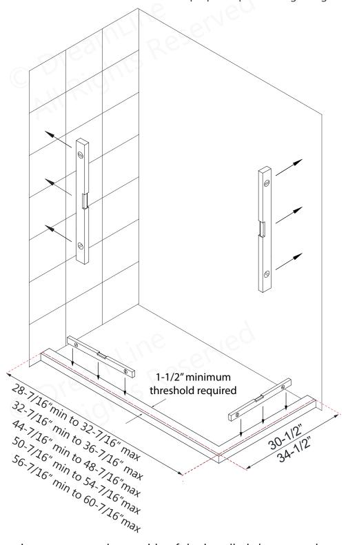
Dimensions represent the outside of the installed shower enclosure (not the dimensions for the shower base or threshold)
