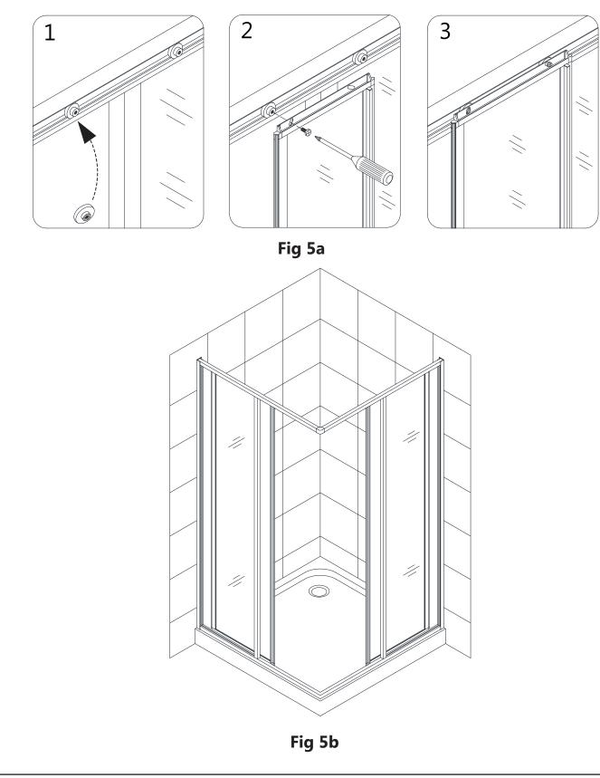
**6.** For smoother operation, if necessary, adjust the position of the **Door Wheels (#11)** within the slot in the **Door Glass (#03)** rail.
