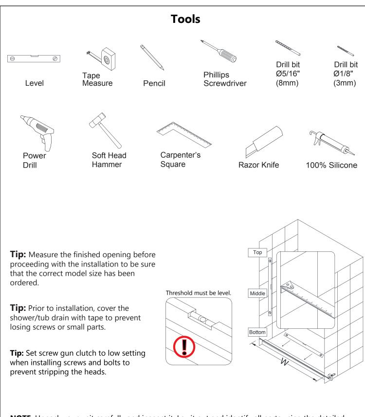
**NOTE:** Unpack your unit carefully and inspect it. Lay it out and identify all parts using the detailed diagram and packing list in this manual as a reference. Before discarding the carton, check for small hardware bags that may have fallen to the bottom of the box. If any parts are damaged or missing, please contact DreamLine<sup>®</sup> for replacement. The shipping boxes may contain extra parts not used in your model configuration.
