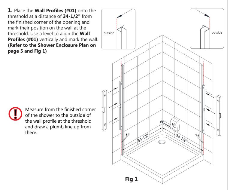
2. Mark the drilling holes on the wall through the predrilled holes in the **Wall Profiles (#01)**. Drill the holes in the wall using a Ø5/16" drill bit and insert the **Wall Anchors (#09)**. Run a bead of silicone along the back surface of the **Wall Profiles (#01)** and around the holes in the wall. Attach the **Wall Profiles (#01)** to the wall using the **Truss Head Screw ST4.2×30 (#05)**. (Fig 2)
