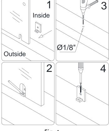
5. Place the **Stationary glass (02)** back into the **Wall profile (01)** and assemble the **Bottom bracket (14)**.
